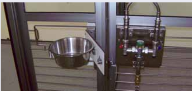
Food bowl hatch located at different heights for variation, only the lower one would be used for minipigs. It is easy to fill the food bowl from outside and swing it back into the pen.
