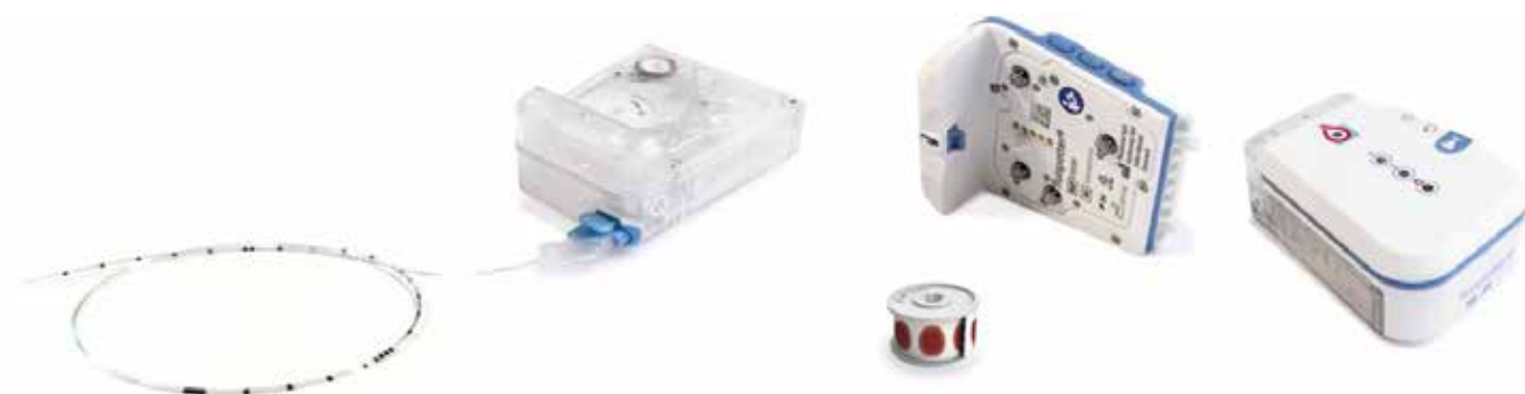
Figure 1 From left: Fluispotter Catheter with markings, attached to Fluispotter Cartridge. Fluispotter Control Unit and to far the right the assembled Fluispotter. In front, paper-reel with dried blood spot samples.
