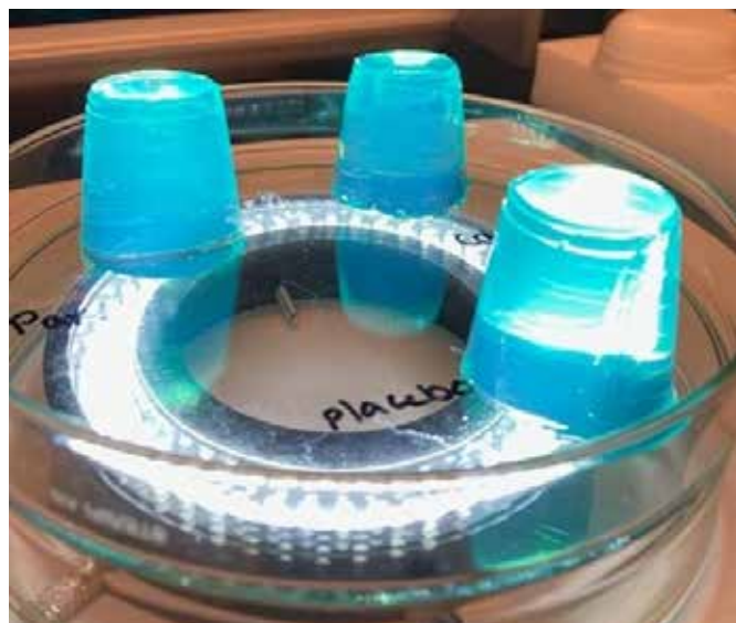
Figure 1 Three oral gelatin formulations evaluated for potential precipitation of compound on a light-box.
