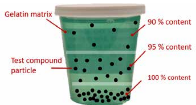
Figure 3 Compound dispersed as solid particles (non-dissolved) in a gelatin matrix. The illustration demonstrates the sedimentation of compound at the bottom, i.e., as an inhomogeneous suspension.
